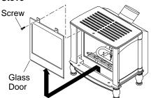
Figure 50 - Removing Glass Door from Burner System Insert Continued
